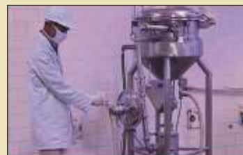
Ointment homogenizer for uniform and homogenous dispersion of active ingredients in every part of ointment.
