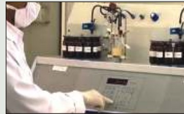
Computer controlled potentiizer to ensure uniform percentage of medicament in each drop.
