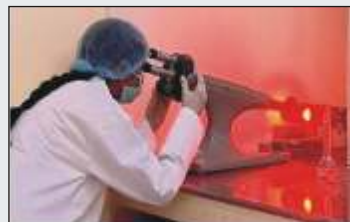
Polarimeter helps to test purity of Lactose
