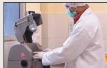
Infrared Moisture Analyzer helps to analyse the moisture in herbs
