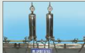
The imported 0.02 Millipore Micron Filter used to avoid any kind of impurities and contamination.
