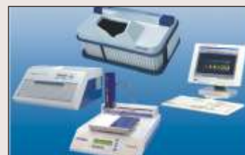
The High Performance Thin Layer Chromatography equipment for qualitative & quantitative analysis
